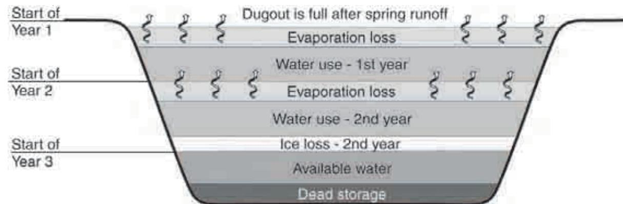
*Supply of available water is reduced by farm use, lack of runoff, evaporation, and ice formation.*
